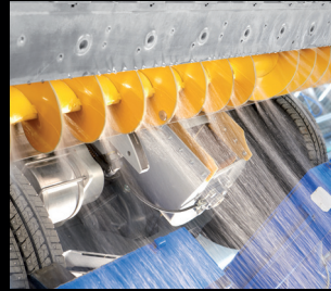
Screw conveyor wash system horizontal
