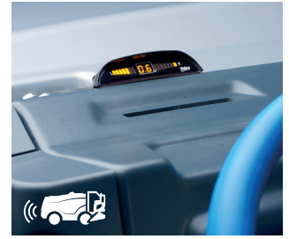
Acoustic distance warning system front
