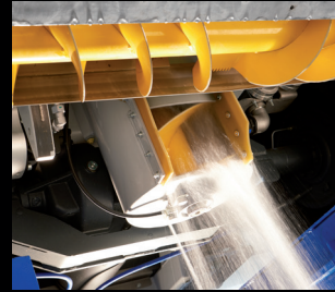
Screw conveyor wash system vertical
