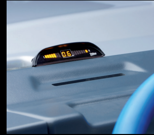
Acoustic distance warning system front
