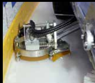
Edger in galvanised steel, electric height adjustment
