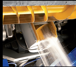
Screw conveyor wash system vertical
