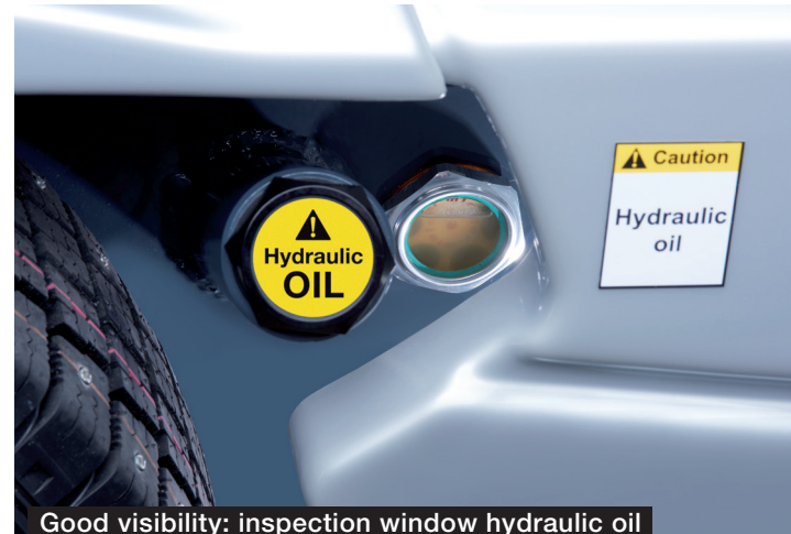
Good visibility: inspection window hydraulic oil
