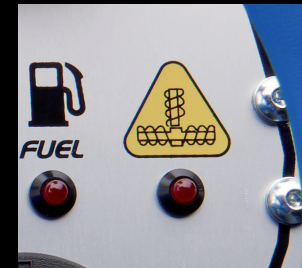
Conveyor screw overload warning system
