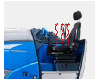
Driver's seat heating Seat pad and backrest
