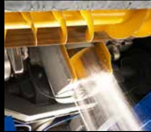
Screw conveyor wash system vertical
