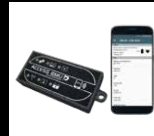
Access BMU Battery-Monitoring-Unit
