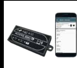
Access BMU Battery-Monitoring-Unit
