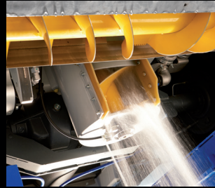
Screw conveyor wash system vertical
