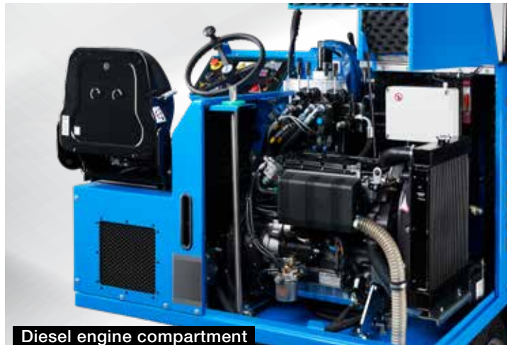
Diesel engine compartment
